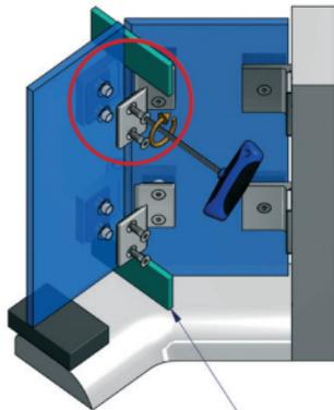
6mm Glaserklötzchen um ein Anschlagen der Gläser bei der Montage zu verhindern. Diese stellen zugleich das Abzugsmaß sicher. | 6mm blocks used by glaziers in order to prevent undesired glass contact during installation. At the same time, the tiny blocks ensure the perfect alignment during measurement due to the proper deduction indicated by the corresponding thickness of the blocks themselves.
